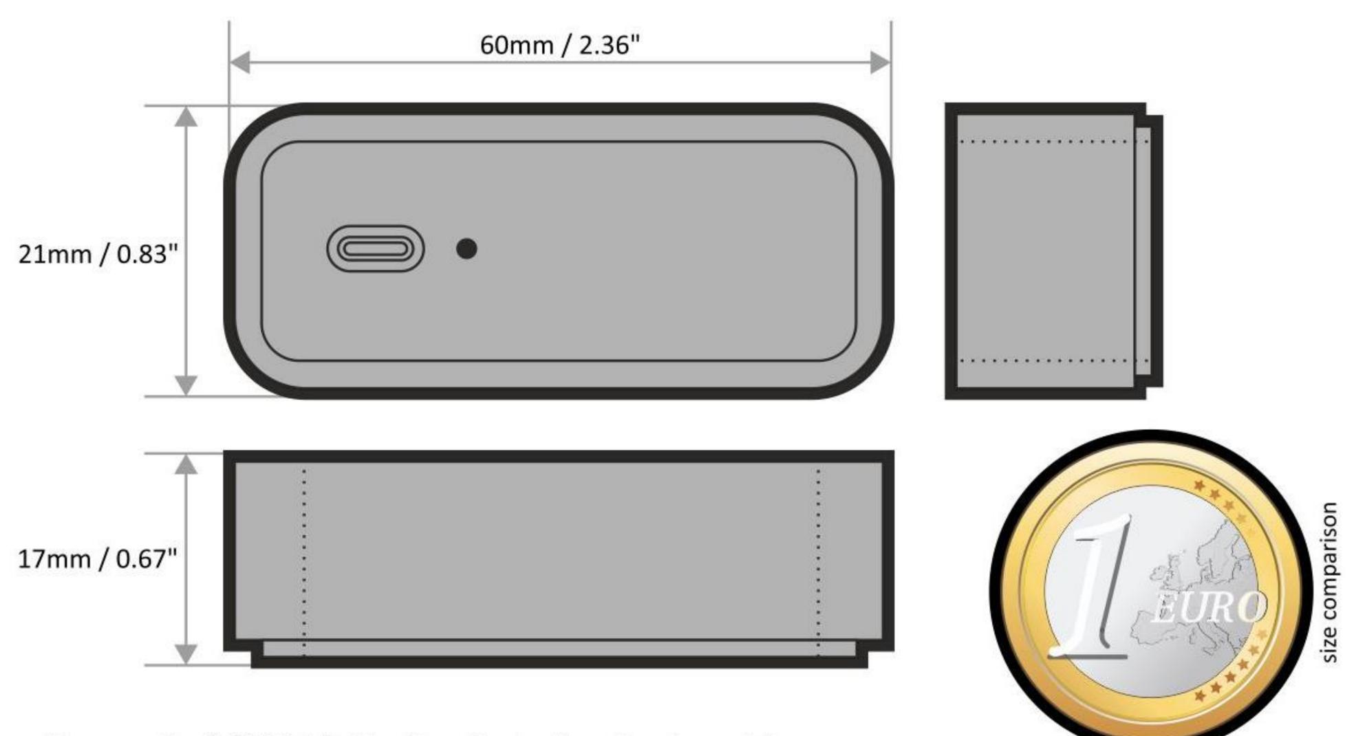
Power: 2x 1.5V AAA Alcaline Batteries. Replaceable. Connectigity: Single Band W-Fi (2-4GHz; 802.11 b/g/n)> Weight: 36 Gramm / 1,27 oz
